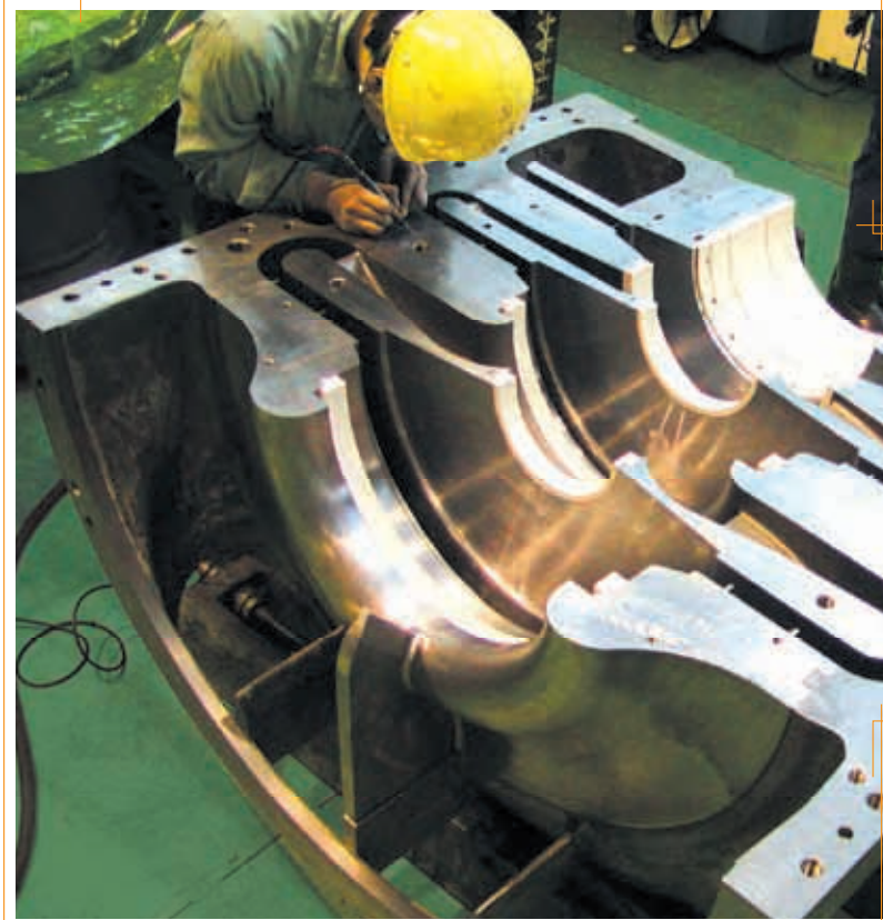
Assembly of an Abradable Seal-Mounted Compressor
