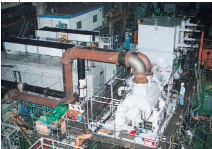
BCH804 Complete Unit Test with 35MW Motor
